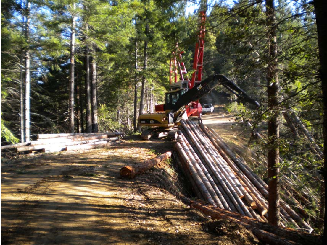
2013 Photo Point 1. WRP timber harvest; yarder and heel boom loader.
